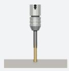
Spot face, drill, and tap a hole with  $\frac{1}{4}$ -28 or M6x1 threads at the desired mounting location.
